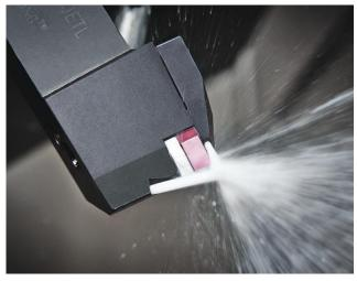
Seco's Jetstream Tooling controls heat and manages chips, preventing hazardous production-stalling tangles while doing away with the hoses and connectors generally required for coolant-through tooling. (Provided by Seco Tools)
