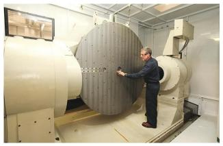
Mitsui Seiki's Wayne Wentworth stands in the work area of a five-axis Mitsui Seiki trunnion machining center. The table was custom engineered to accommodate a 78" (198-cm) diameter part. (Provided by Mitsui Seiki)
