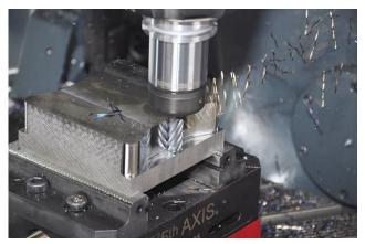
Optimized roughing with Seco's Niagara Cutter multi-flute end mill. The tool is designed for chip control in applications requiring depths of cut up to 3X tool diameter. (Provided by Seco Tools)
