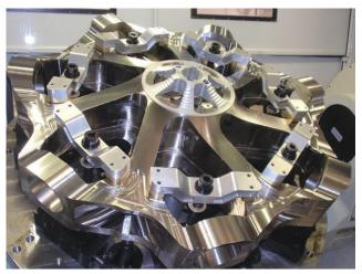
Prismatic workpieces such as this helicopter rotor hub are typical work for Mitsui Seiki's large five-axis machining centers. (Provided by Mitsui Seiki)
